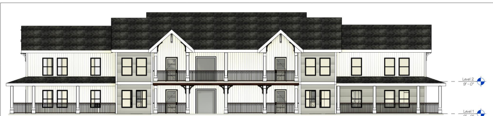
3 A3.2 SCALE: 1/8" = 1'-0" BLDG. B (2-STORY) REAR ELEVATION
